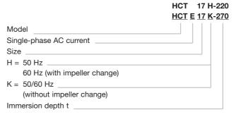
Please indicate electrical parameters, e.g. 230/400 V, 50 Hz. When ordering spare parts, always indicate the 10-place serial number (see motor rating plate).
