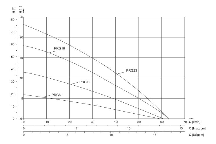
The data apply to fluids with a viscosity of 1 mm<sup>2</sup>/s at a density of 1 kg/dm<sup>3</sup>
