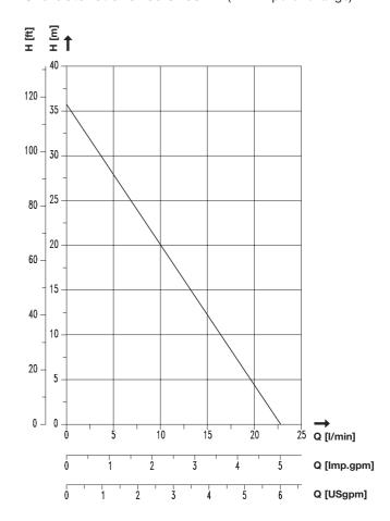
The data apply to fluids with a viscosity of 1 mm<sup>2</sup>/s at a density of 1 kg/dm<sup>3</sup>
