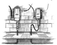
Standpipe and wall mount assembly to remote bulk tanks
