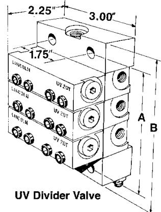
UV Divider Valves are designed to meter oil or grease in automatic or manual systems installed on all types of industrial machinery. Segmented baseplate assembly contains all inlet and outlet connections. Alternate outlet ports are located on the face of the divider valve which may be used for installation of performance indicators.
