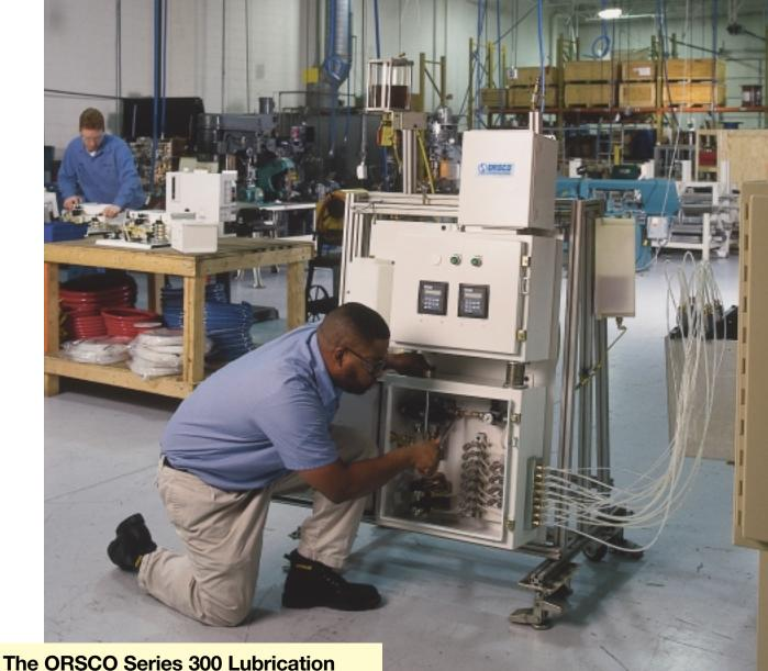
The ORSCO Series 300 Lubrication System provides complete monitoring of both air and oil lines for 100 percent delivery verification.
